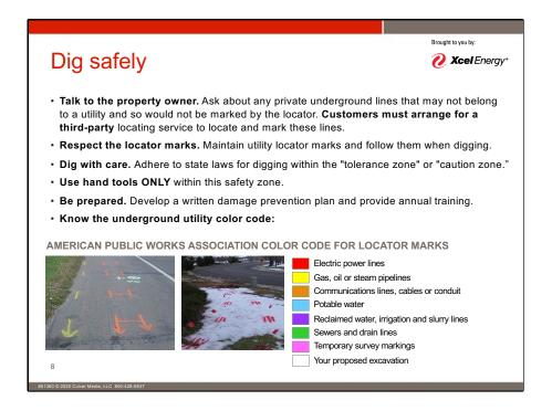
Dig safely. After you call 811 or place an online ticket request, the underground utility locator service will arrange for each utility to send someone out to mark underground lines.
